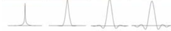
FIGURE 4.44 (a)-(d) Spatial representations of Butterworth low-pass filters of orders 1, 2, 3, and 4, and corresponding intensity profiles through the center of the filters (the size is all cases is 1000 x 1000 and the cutoff frequency is 5). Observe how ringing increases as a function of filter order.
