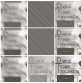
FIGURE 5.29 (a) 8-bit image corrupted by motion blur and additive noise. (b) Result of inverse filtering. (c) Result of Wiener filtering. (d)–(f) Same sequence, but with noise variance one order of magnitude less. (g)–(i) Same sequence, but noise variance reduced by five orders of magnitude from (a). Note in (h) how the deblurred image is quite visible through a “curtain” of noise.
