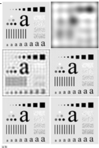
FIGURE 4.43 (a) Original image. (b)-(i) Results of filtering using LLPFs with small variations of radii. (b) 5, (c) 10, (d) 15, (e) 20, (f) 25, (g) 30, (h) 35, (i) 40. The images are arranged in the order (a), (b), (c), (d), (e), (f), (g), (h), (i).
