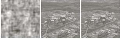
FIGURE 5.28 Comparison of inverse and Wiener filtering. (a) Result of full inverse filtering of Fig. 5.25(b). (b) Radially limited inverse filter result. (c) Wiener filter result.
